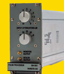
Module (94 series) The building blocks of the architecture is a catalogue of 3U-high modules, designed to perform a given functional task.
