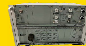
Unit (95 series) Configurable sub-systems of modules, mounted in 19-inch chassis, in 3U or 6U configurations.
