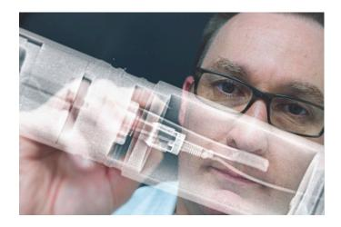
AGRs create a particularly hostile environment for neutron detectors, which must withstand the very high temperature that is a characteristic of them. While detectors can operate to design specification for decades, at some point their performance will degrade.
